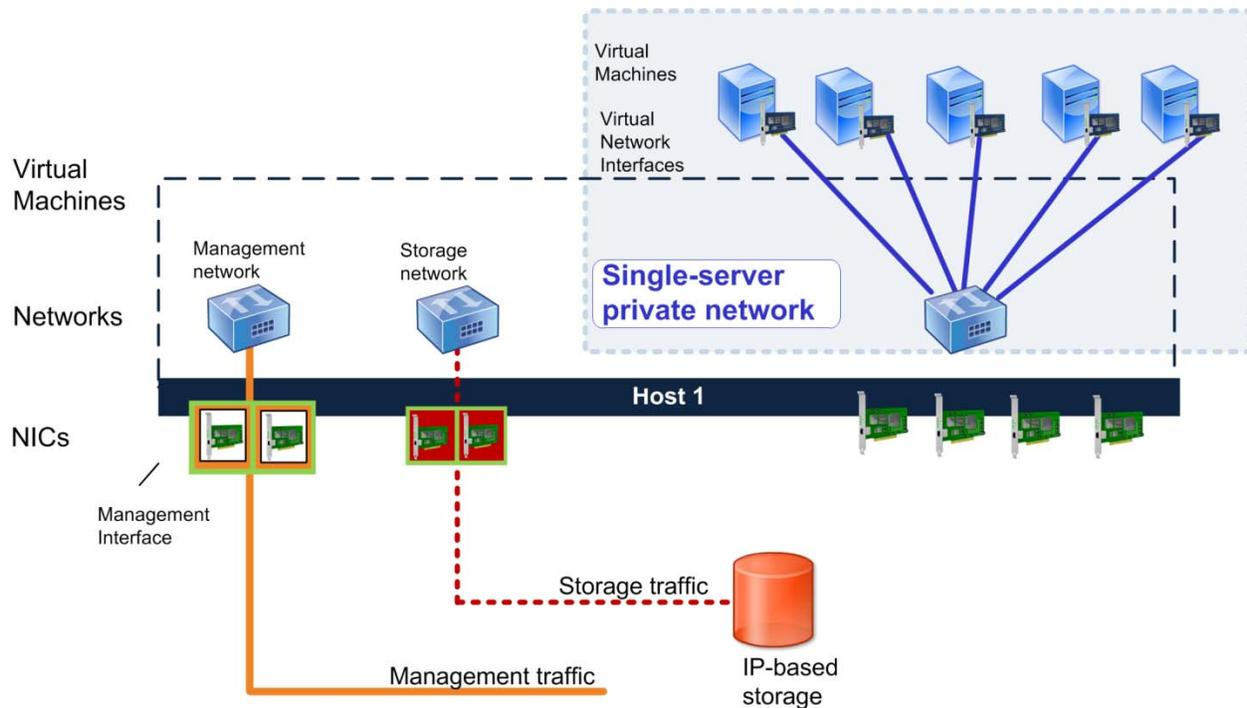
*This illustration shows how the virtual network interfaces on the VMs are on the single-server private network. This network does not have any connect to any NICs since all traffic is sent inside the XenServer host.*
