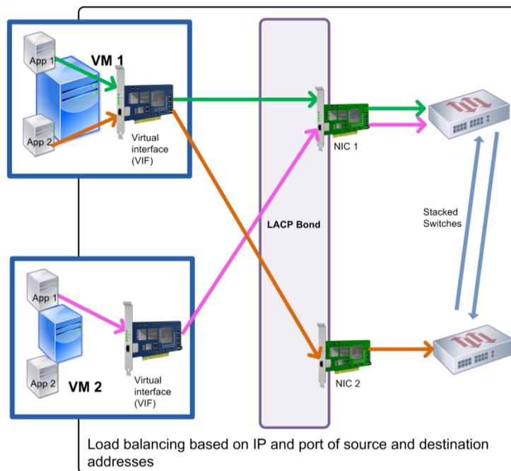
*This illustration shows how, if you use LACP bonding and enable **LACP with load balancing based on IP and port of source and destination** as the hashing type, the traffic coming from two different applications on VM1 can be distributed to two NICs*
