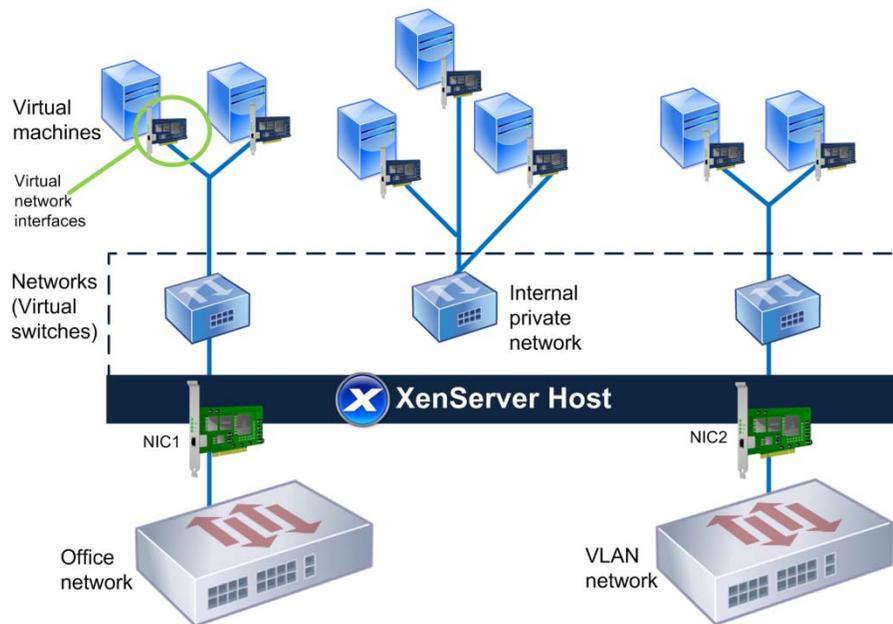
*The VMs connect to three different types of networks: an office network, an internal private network, and a VLAN.*
