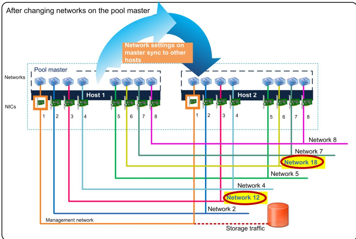
These two illustrations show how XenServer replicates the network settings created on the pool master on all other hosts in the pool. In the top illustration, NICs 3 and 6 on both hosts use Networks 3 and 6. In the bottom illustration, after reconfiguring NIC 3 on the pool master to use Network 12 and NIC 6 to use Network 18, XenCenter automatically configures the other host in the pool to use those settings.
