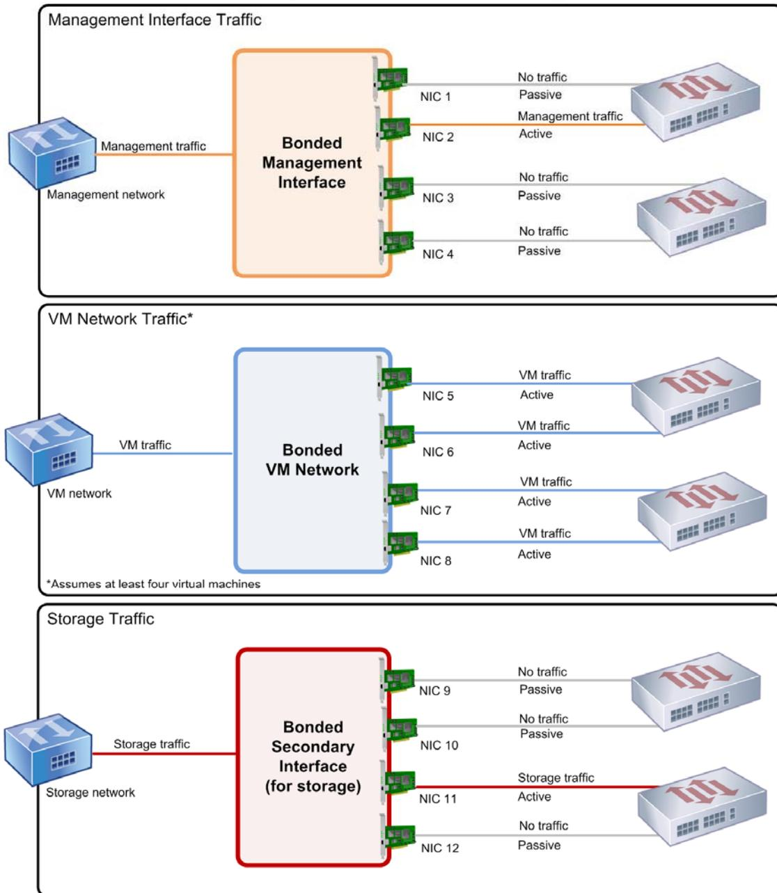
*This illustration shows how bonding four NICs may only benefit guest traffic. In the top picture of a management network, NIC 2 is active but NICs 1, 3, and 4 are passive. For the VM traffic, all four NICs in the bond are active; however, this assumes a minimum of four VMs. For the storage traffic, only NIC 11 is active.*
