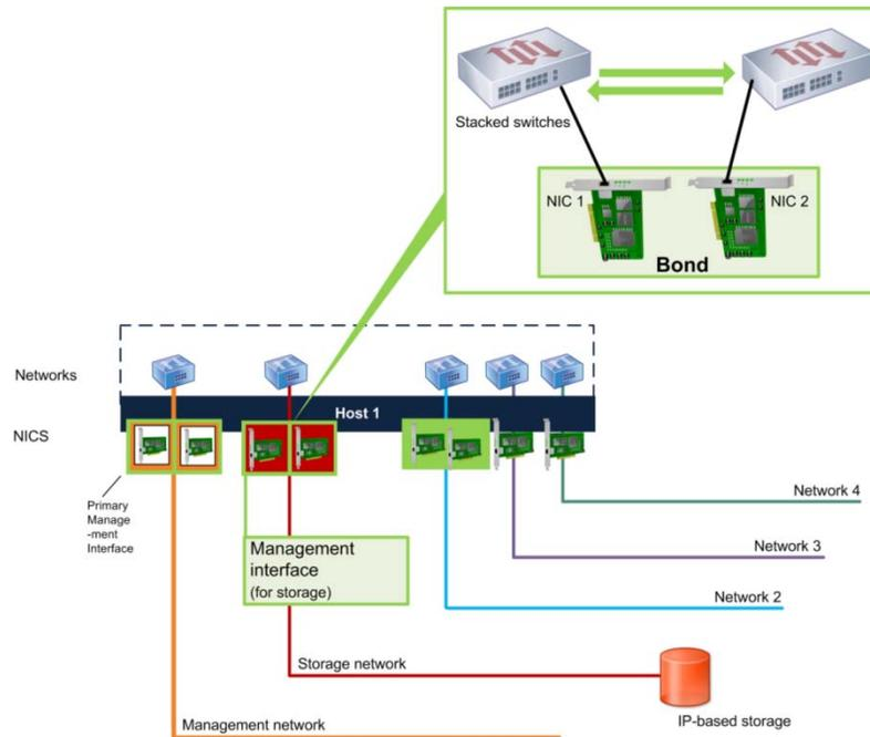
*This illustration shows how the bond made from NICs 3 and 4 is configured as a secondary interface. XenServer sends its storage traffic over this NIC bond onto the storage network and, ultimately, the storage array. The exploded diagram shows how each NIC in the bond connects to a different switch. Note: The need for stacked switches varies according to the bond mode. See page **Error! Bookmark not defined.***
