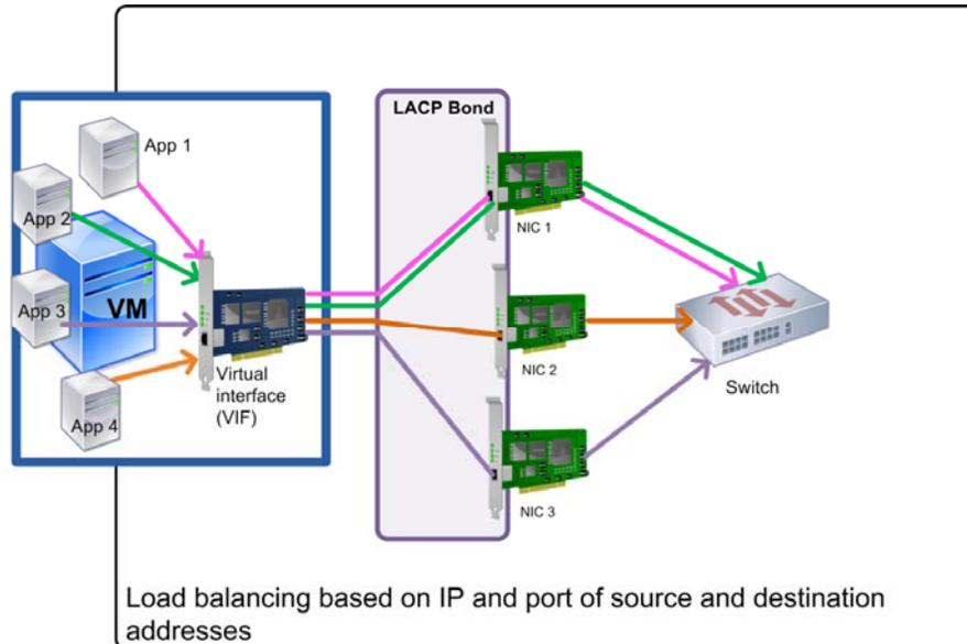
*This illustration shows how, if you use LACP bonding and enable **LACP with load balancing based on IP and port of source and destination** as the hashing type, XenServer can send the traffic of each application in the virtual machine through one of the three NICs in the bond even though the number of NICs exceeds the number of virtual network interface.*
