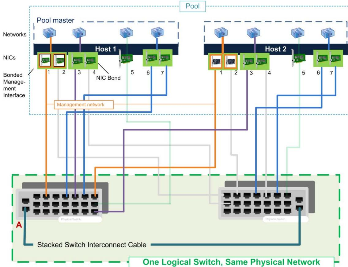
*This illustration shows two stacked switches connected with the vendors proprietary interconnect cable across the same physical network. These switches function logically as one unit. Because there are no VLANs configured on any of the ports and all ports have the same connectivity, the NICs can be plugged into any port on these two switches. Note: The need for stacked switches varies according to bond mode, as described on page **Error! Bookmark not defined.***
