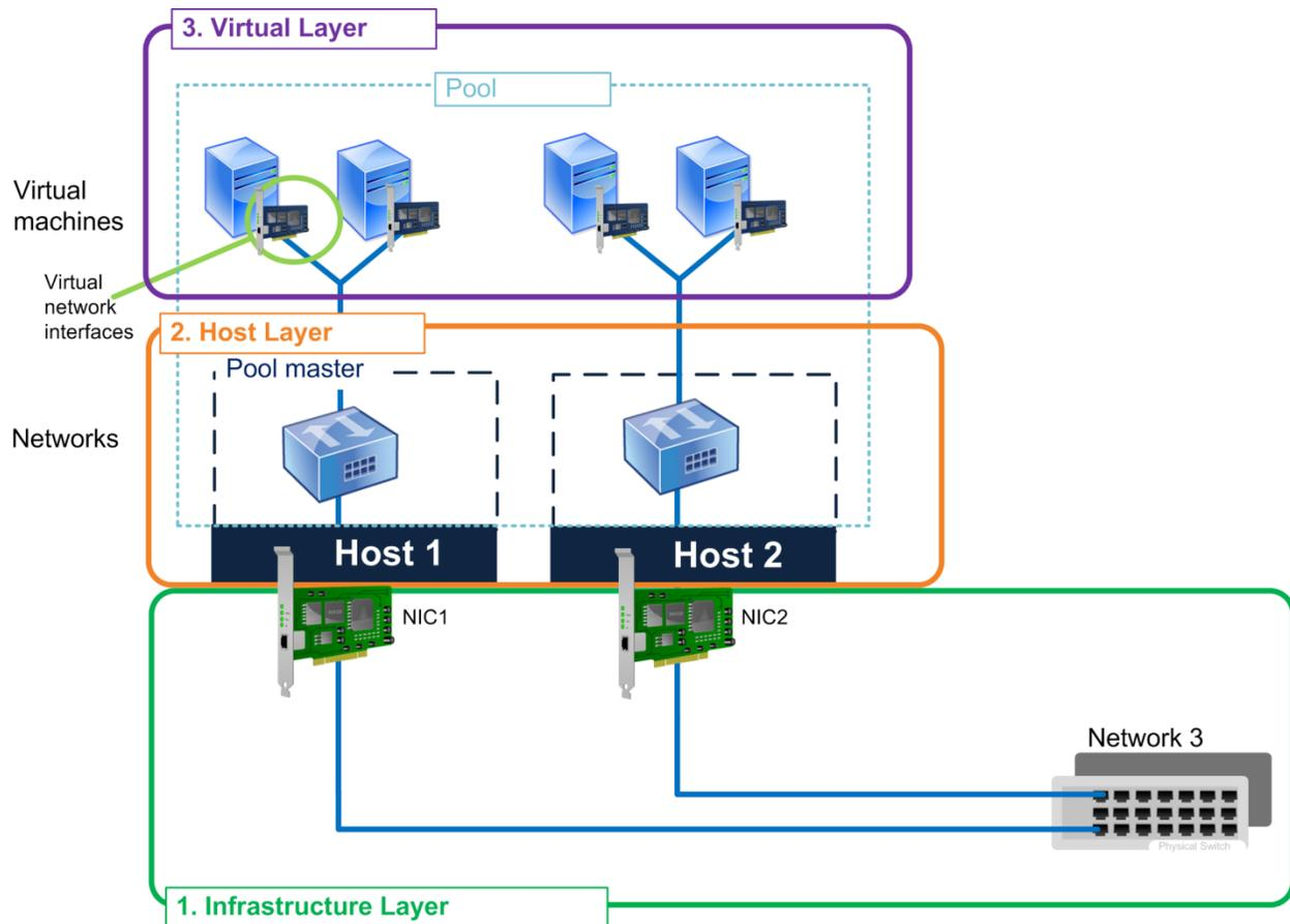
*This illustration shows the order in which you should configure networking in your virtual environment: (1) Start on the physical infrastructure layer, which means connecting NICs to switches; (2) configure the hardware layer, which means connecting hosts to networks and configuring these networks; (3) configure the virtual layer, which means attaching VMs to networks through virtual network interfaces.*
