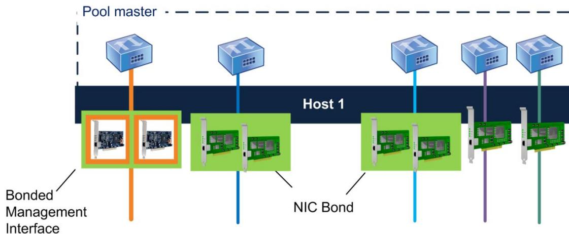
*This illustration shows three pairs of bonded NICs, including the management interface. Excluding the management interface bond, in this example, XenServer uses the other two NIC bonds and the two un-bonded NICs for VM traffic.*
