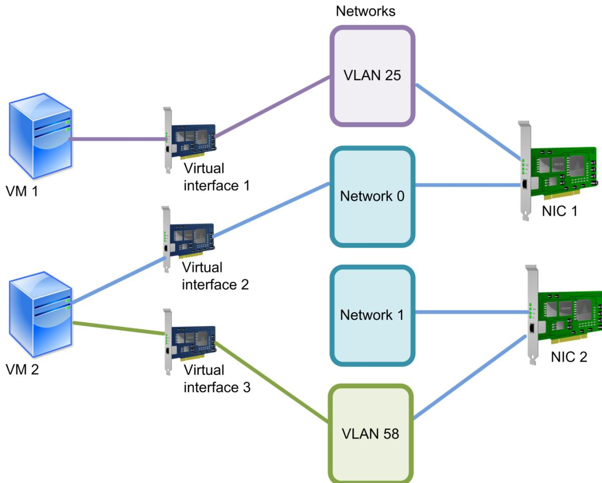
*This illustration shows how VMs require a separate virtual network interface for each network to which you want to connect them, including VLANs. In this example, VM 2 connects to Network 0 through Virtual Network Interface 2 and to VLAN 58 through Virtual network interface 3. As shown by VM1 and NIC1, multiple networks can connect out through one NIC.*
