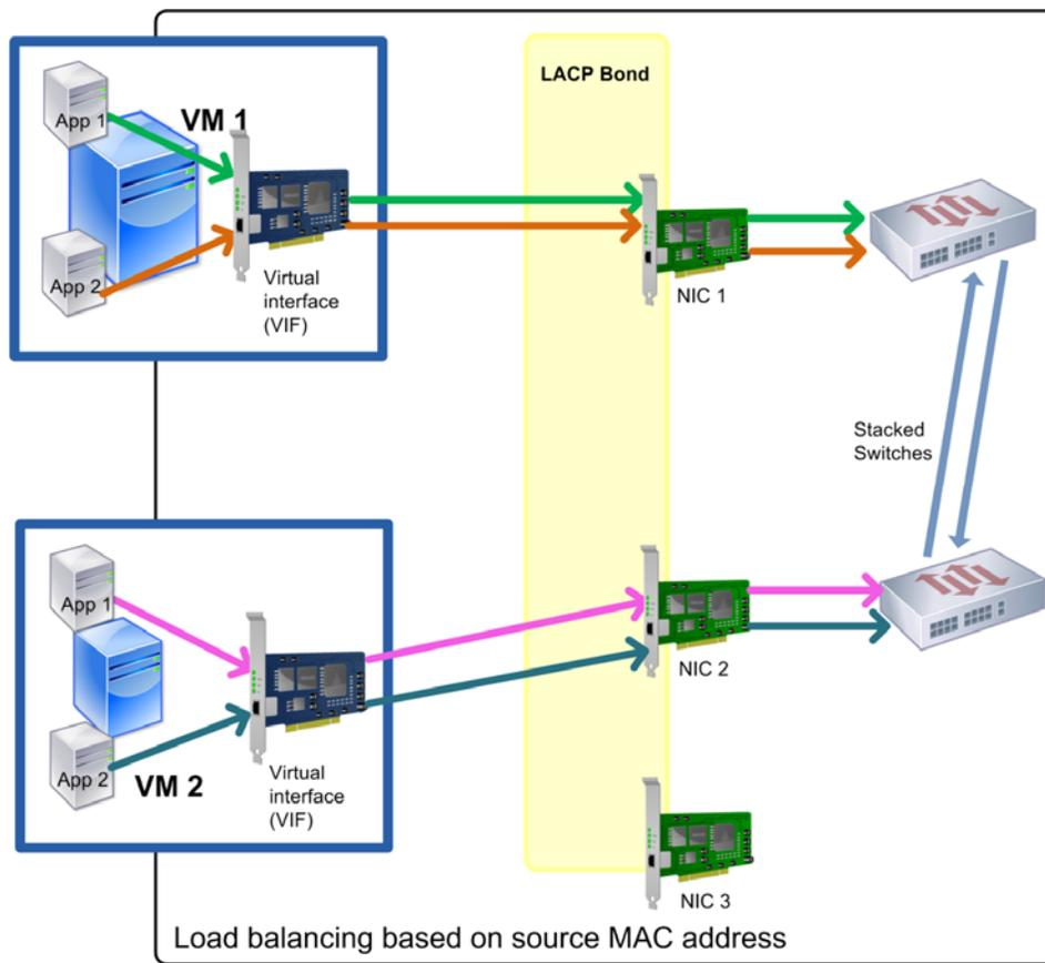
*This illustration shows how, if you use LACP bonding and enable LACP based on source MAC address as the hashing type, if the number of NICs exceeds the number of virtual network interfaces, not all NICs will be used. Because there are three NICs and only two VMs, only two NICs can be used at the same time and the maximum bond throughput cannot be achieved. The packets from one VM cannot be split across multiple VMs.*
