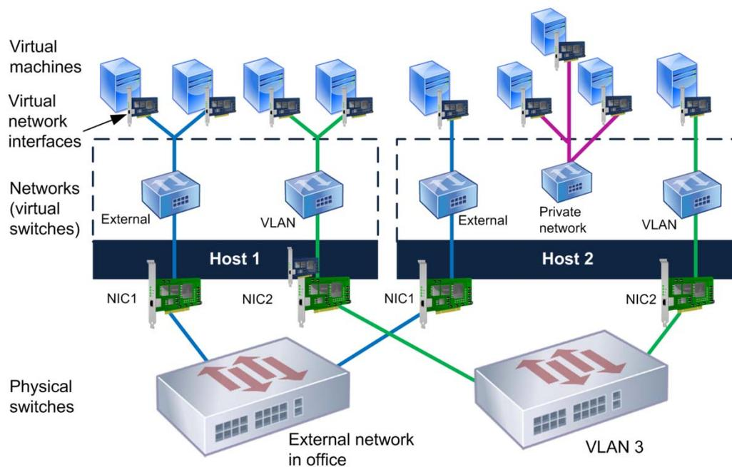
*This illustration shows how virtual machines connect to three different types of networks: an external network, a VLAN network, and a single-server private network.*
