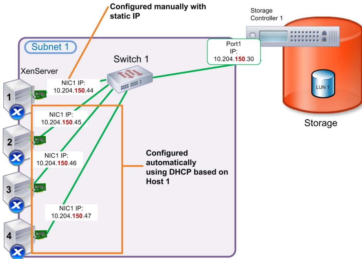
*This illustration shows how after an administrator created a secondary interface on NIC 3 on Host 1 and set it to 10.204.150.44, XenServer automatically created secondary interfaces on the other hosts in the pool and set their IP addresses using DHCP. Each host in the pool is assigned the next IP address in the range –Host 2 is set to 10.204.150.45, Host 3 is set to 10.204.150.46, and Host 4 is set to 10.204.150.47.*
