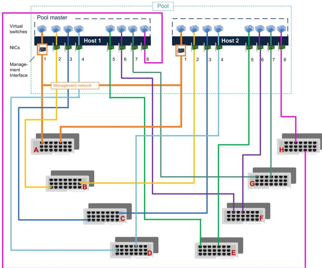
*This illustration shows how each corresponding NIC on both hosts must physically connect to the same network. Each switch represents a separate physical network. Each member host's NICs must be connected to the same physical networks as the corresponding NICs on the pool master.*
