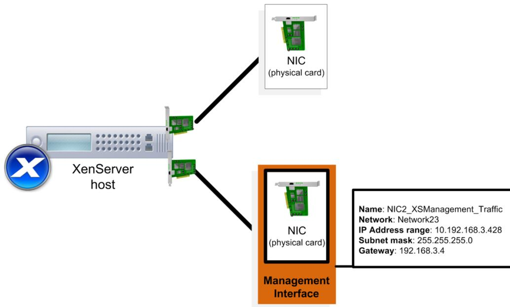
*This illustration contrasts a regular NIC with one configured as the management interface. The management interface has an IP address, subnet mask, and gateway assigned to it.*
