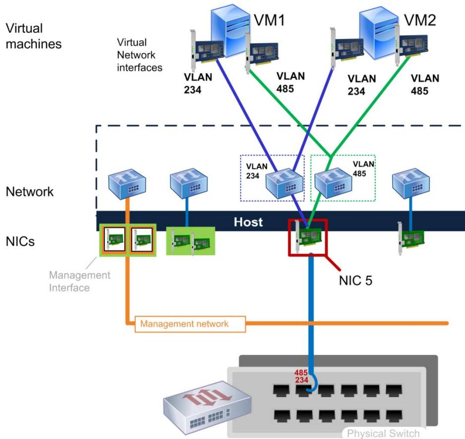
*This illustration shows how VMs on the host connect to an external network that the administrator configured to connect to VLAN 485 and VLAN 234. To achieve this, the administrator created an external network that uses NIC 5 to connect to a trunked switch port that includes VLAN 485 and a second external network that also uses NIC 5 to connect to VLAN 234. The administrator ran a cable from the VLAN trunk port to NIC 5.*
