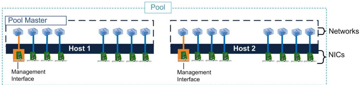
*This illustration shows two hosts joined together in a pool before any networking configuration is performed on them.*
