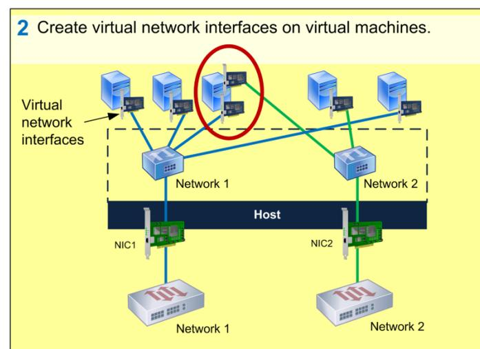
*This illustration shows how VMs require a virtual network interface for each physical network to which they need to connect.*
