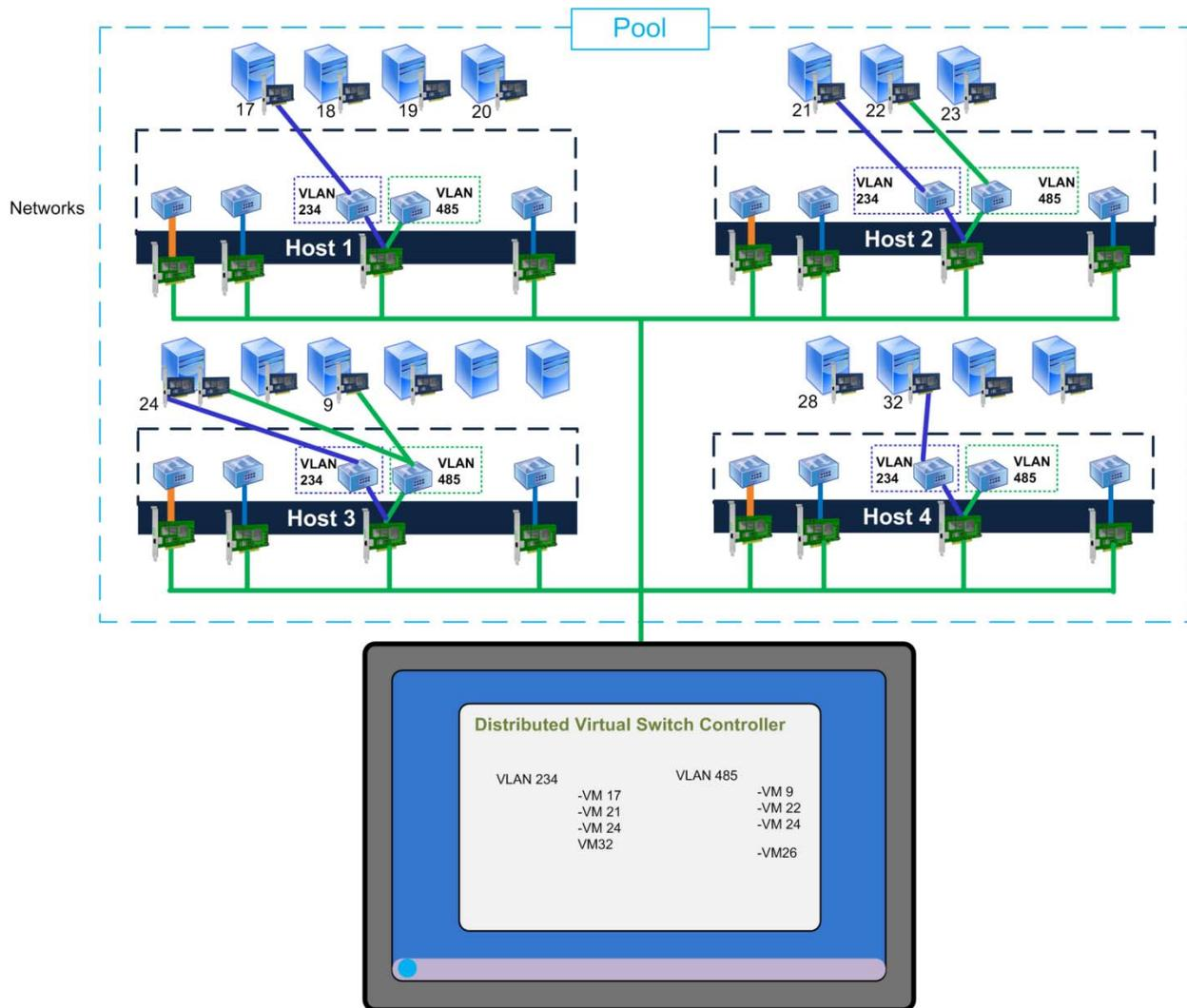
*This illustration shows how the vSwitch Controller can display which VLANs are used by which virtual machines and let you display these VLANs from one central user interface.*
