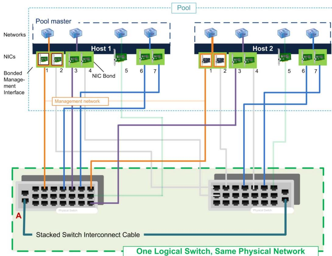
*This illustration shows how two NICs in a bonded pair (LACP bond mode) use the same network settings, as represented by the networks in each host. The NICs in the bonds connect to two stacked switches for redundancy.*
