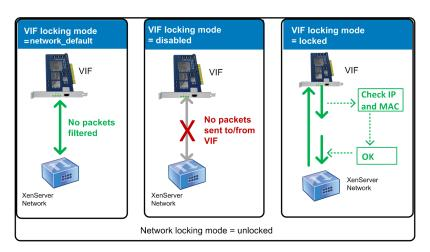
This illustration shows how three different VIF locking mode states behave when the network locking mode is set to unlocked and the VIF state is configured. In the first image, the VIF state is set to default so no traffic from the VM is filtered. In the second image, the VIF does not send or receive any packets because the locking mode is set to disabled. In the third image, the VIF state is set to locked, so the VIF can only send packets if those packets contain the correct MAC and IP address.
