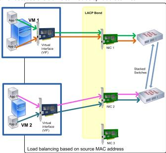
This illustration shows how, if you use LACP bonding and enable LACP based on source MAC address as the hashing type, if the number of NICs exceeds the number of VIFs, not all NICs will be used. Because there are three NICs and only two VMs, only two NICs can be used at the same time and the maximum bond throughput cannot be achieved. The packets from one VM cannot be split across multiple VMs.
