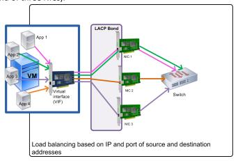
This illustration shows how, if you use LACP bonding and enable LACP with load balancing based on IP and port of source and destination as the hashing type, XenServer can send the traffic of each application in the virtual machine through one of the three NICs in the bond even though the number of NICs exceeds the number of VIFs.
