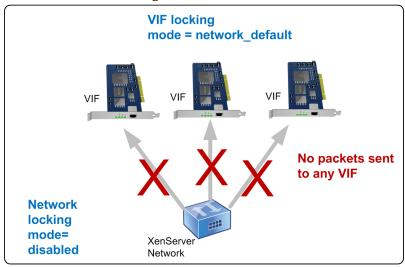
This illustration shows how a VIF, when configured at its default setting (locking-mode=network\_default), checks to see the setting associated with the default-locking-mode. In this illustration, the network is set to default-locking-mode=disabled so no traffic can pass through the VIF.
