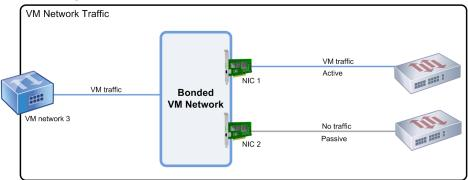
This illustration shows two NICs bonded in active-passive mode. NIC 1 is active. The bond includes a NIC for failover that is connected to a second switch. This NIC will be used only if NIC 1 fails.
